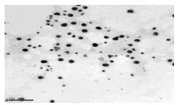
Figure 3: The HRTEM image shows gold nano particles of a maximum of 30 nm size. Mostly spherical AuNPs were observed along with certain percentage of triangular shaped particles.
