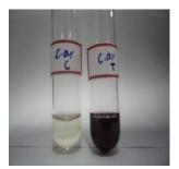
The synthesized gold nanoparticles were characterised using UV-visible spectroscopy, The optical properties of metal nanoparticles are dominated by surface Plasmon resonance (SPR), which shifts to longer wavelength with increasing particle size <sup>12</sup>. The strong surface Plasmon reference centred at 530nm is the characteristics of colloidal gold (Figure- 2).
