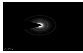
Selected area electron diffraction (SAED) pattern obtained from a AuNPs (Figure- 4) revealed three diffraction rings from inner to outer associated with the [111], [200], and [222] planes of FCC crystalline Au indicating the formation of crystalline gold nanoparticles. The spots are indexed according to FCC structure of Au.
